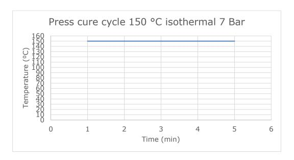
**Pressure:** Minimum of 7 bar (7.2 kg/cm2) (\*), **30 bar is recommended.**
