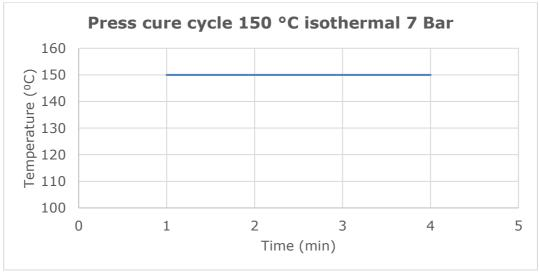
Pressure: Minimum of 7 bar (7.2 kg/cm2) (\*), 30 bar is recommended.
