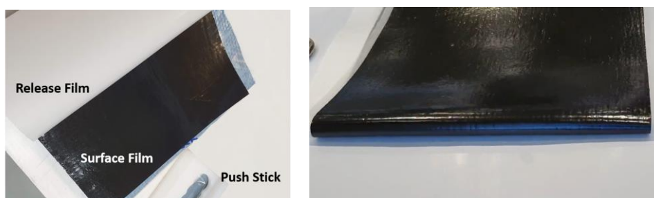
Figure 1 Correct way of laying tooling prepreg on mold surface.
